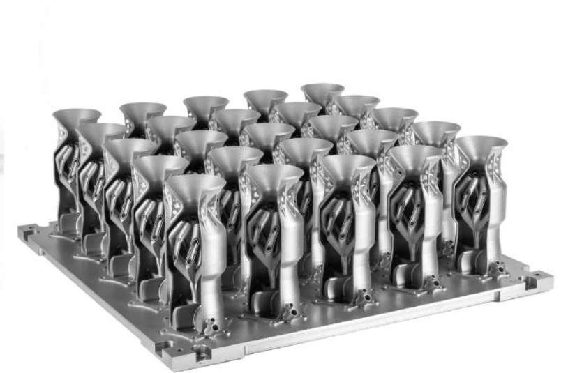
Fuel Injection nozzles
